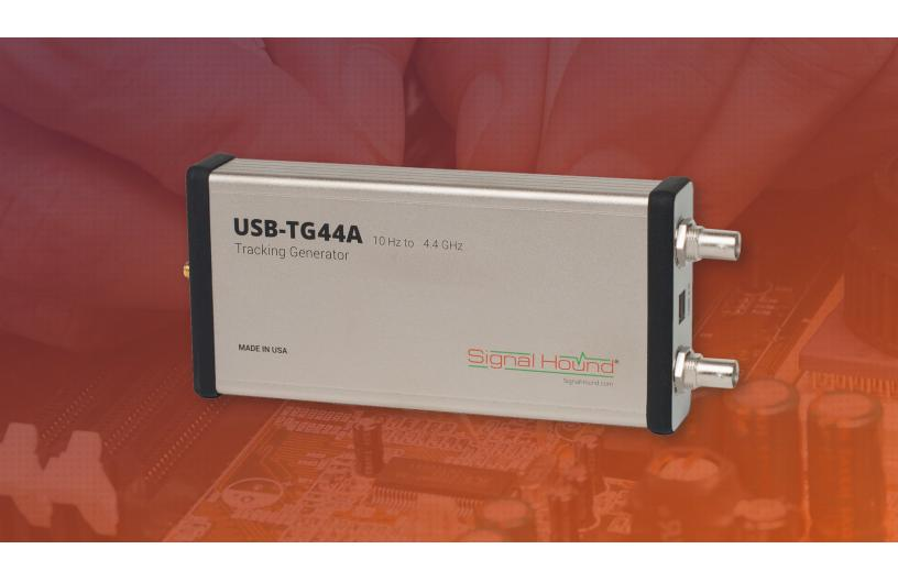
Adds versatile scalar network analysis capability to your USB-SA44B Spectrum Analyzer. Use as a CW Signal Generator for tasks that will tolerate harmonics of typically < -10dBc.
