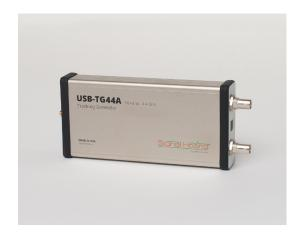
The Signal Hound TG44A is a USB-powered, 10 Hz to 4.4 GHz, economy tracking generator and CW signal generator. The TG44A turns your SA44B, SA124B, or BB60C spectrum analyzer into a versatile scaler network analyzer. The combination can measure gain, frequency response, compression, flatness, and insertion loss on components and subsystems.
